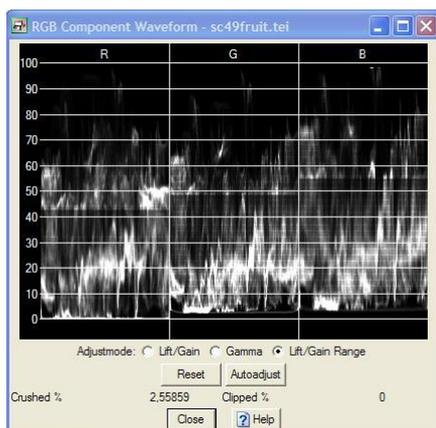
The RGB Wave form displays the wave form for each color separately.
