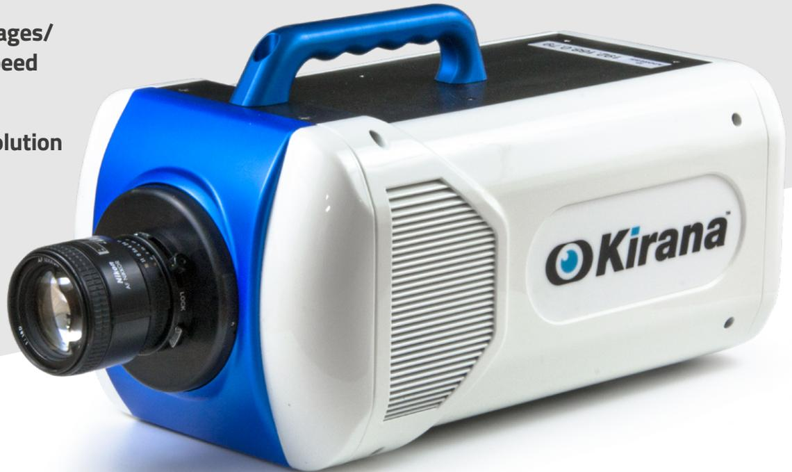
The Specialised Imaging KIRANA is a true Ultra high-speed video camera that combines the flexibility of a video camera with the speed/resolutions approaching those only available with Framing cameras.
